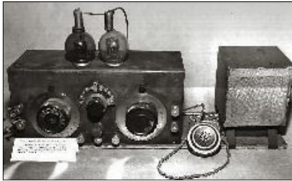
One half of Armstrong's first model, as it was displayed in the Army Communications Museum at Ft. Monmouth, New Jersey in 1980. The right-hand box, the headphone, and the VT2 tubes with the caps resting on them, are all incorrect, but the set has been displayed this way since at least 1954. This model, with its four-tube amplifier box, is shown in its original condition in Radio News, Feb. 1920 (ref.15). U.S. Army photo, courtesy of H.L. Chadbourne.
