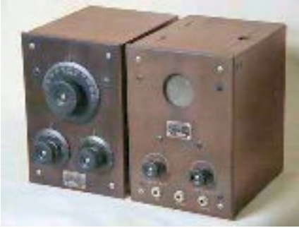
Westinghouse RA tuner and DA detector-amplifier, designed in 1920 by Frank Conrad and Donald Little
