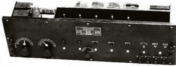
120957. SUPER HETERODYNE RECEIVER MANUFACTURED BY WESTERN ELECTRIC COMPANY, SHOWING PANEL WITH APPARATUS MOUNTED ON REAR. INDEX 654 11 12 23
