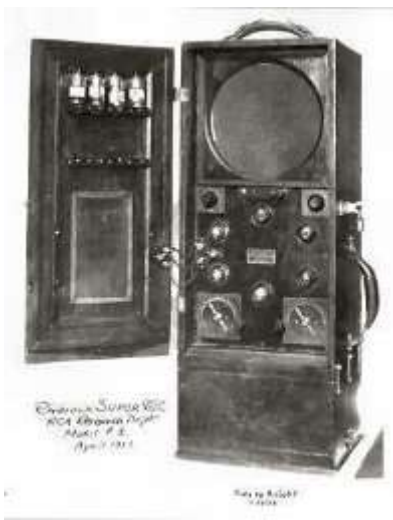
portable superheterodyne; the two models shown had evolved by 1925 into the Radiola 26. Model #2 is now in the Ford Museum.
